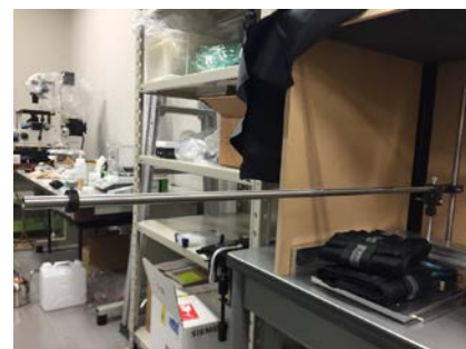
Figure 4: load application device before introducing force test stand. The horizontal bar is the leverage.
